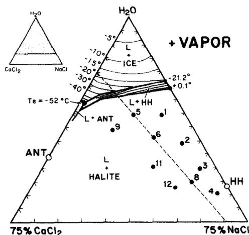
FIG. 1. Phase diagram for part of the ternary system NaCl-CaCl<sub>2</sub>-H<sub>2</sub>O, after YANATIEVA (1946). Compositions are in weight percent. Ternary eutectic is at about -52°C. ANT is antarcticite and HH is hydrohalite. Solid dots show bulk compositions of synthetic fluid inclusions in this study, and their sample numbers. The dashed line shows the join between (H<sub>2</sub>O)<sub>80</sub>-(CaCl<sub>2</sub>)<sub>20</sub> and NaCl that is drawn in Fig. 5.
