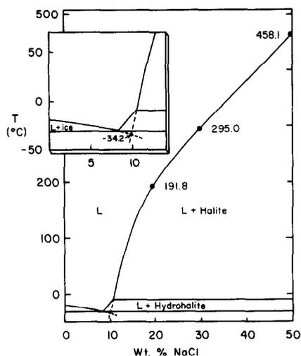
FIG. 5. Portion of the pseudobinary section of the ternary system NaCl-CaCl<sub>2</sub>-H<sub>2</sub>O varying from a composition of 80 wt% H<sub>2</sub>O, 20 wt% CaCl<sub>2</sub> (*i.e.*, 0% NaCl) to 100% NaCl (see Figs. 1 and 3 for location). Temperatures labelled on the liquidus have been determined in the present study, as has the temperature of ice melting in the presence of metastable halite (-34.2°C). The ice and hydrohalite liquidus curves are interpolated from data of YANATIEVA (1946).
