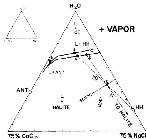
FIG. 4. Liquid line of descent for a bulk liquid composition at point a, which corresponds to sample 2 (39.6% NaCl, 6.0%  $\text{CaCl}_2$ , 54.4%  $\text{H}_2\text{O}$ ). The path is discussed in the text. Triangles are the inferred natural compositions from Mathematician Ridge fluid inclusions (Table 3).
