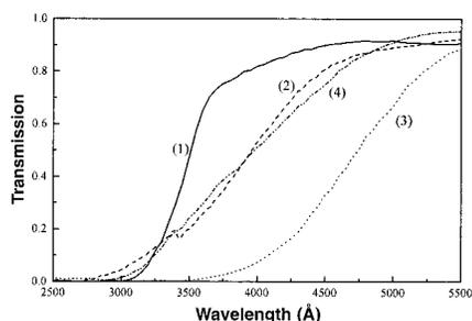
**Fig. 4.** The UV spectra of different SnO<sub>2</sub> materials. (1) Micrometer-sized crystals obtained from oxidation of tin at 1000°C; (2) H-gel fired at 500°C for 1 hour; (3) U-gel fired at 500°C for 1 hour; and (4) U-gel fired at 800°C for 1 hour.
