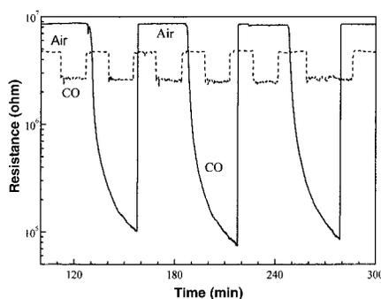
**Fig. 5.** The response curves of CO sensors made of Pd-impregnated U-SnO<sub>2</sub> (dashed line) and H-SnO<sub>2</sub> (solid line) films at 20°C.
