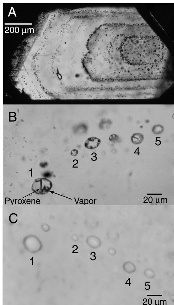
FIG. 3. A. Photomicrograph of orthopyroxene crystal showing several growth surfaces outlined by melt and mineral inclusions. B. Crystallized (type IV) melt inclusions in plagioclase from the 1991 eruption. Each inclusion contains a pyroxene crystal and a vapor bubble. C. Same area shown in (B) after heating the inclusions to homogenization followed by quenching to glass.
