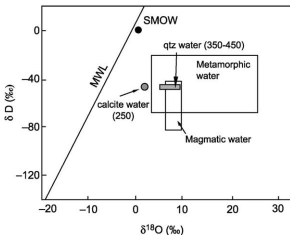
Fig. 6. Plot of measured  $\delta\text{D}$  vs calculated  $\delta^{18}\text{O}$  for water in equilibrium with hydrothermal quartz at 350–450 °C (shaded box). The shaded circle represents the calculated oxygen isotopic composition of water in equilibrium with calcite at 250 °C. Also shown are the metamorphic and magmatic water boxes from Taylor (1979). MWL = Meteoric Water Line. SMOW = Standard Mean Ocean Water.
