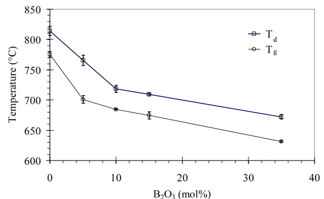
**Fig. 3** Glass transition temperature ( $T_g$ ) and glass softening temperature ( $T_d$ ) variation with  $\text{B}_2\text{O}_3$  content in SABS glasses
