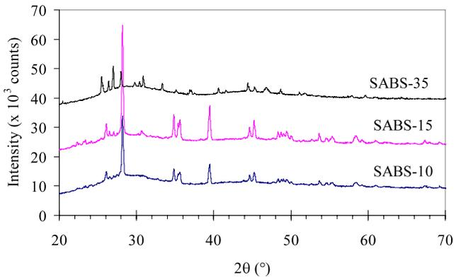
**Fig. 6** XRD patterns of SABS-10, SABS-15, and SABS-35 glasses thermally treated at 850°C for 50 hrs
