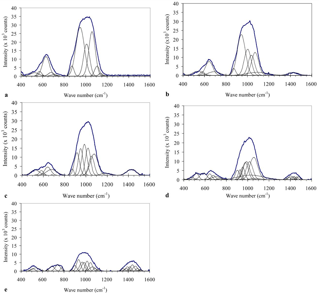
**Fig. 2** Deconvoluted Raman spectra for: (a) SABS-0, (b) SABS-5, (c) SABS-10, (d) SABS-15, and (e) SABS-35 glasses
