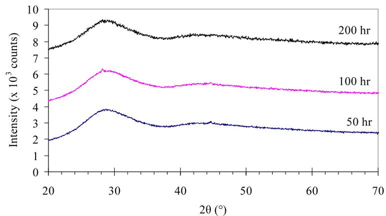
**Fig. 5** XRD patterns of SABS-5 glass thermally treated at  $850^\circ\text{C}$  for different times
