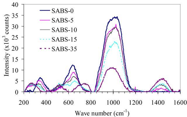
**Fig. 1** As collected Raman spectra of different SABS glasses
