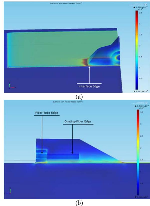
**Figure 6.** The COMSOL® produced stress distribution at 973K for the (a) front of the model and (b) the right side (symmetry plane) view of the model. The maximum of the color range is set to the adhesion strength of the deposit.
