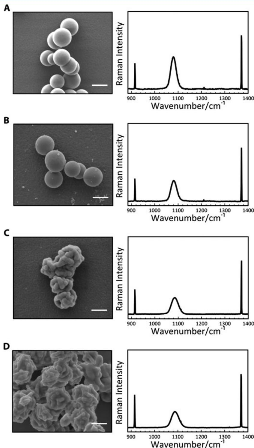
**Figure 1.** Scanning electron microscopy images show the characteristic morphologies of ACC precipitates with the corresponding Raman spectra of carbonate  $\nu_1$  peak (center) and Ne emission lines at  $914.90\text{ cm}^{-1}$  and  $1371.26\text{ cm}^{-1}$ . (a) ACC that contains 0 mol %  $\text{MgCO}_3$ ; (b) ACC with 10 mol %  $\text{MgCO}_3$ ; (c) ACC with 34 mol %  $\text{MgCO}_3$ ; and (d) ACC with 43 mol %  $\text{MgCO}_3$ . All scale bars =  $1\ \mu\text{m}$ .
