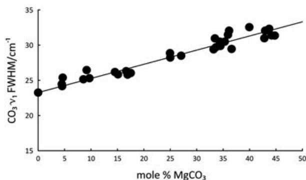
**Figure 3.** Carbonate  $\nu_1$  FWHM versus  $\text{MgCO}_3$  content (mol %) of ACC. Line represents least squares fit with an  $R^2$  value of 0.946.
