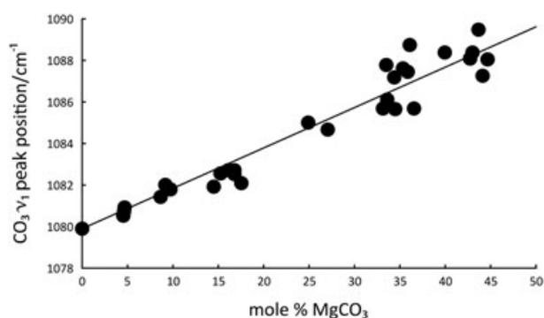
**Figure 2.** Carbonate  $\nu_1$  peak position versus  $\text{MgCO}_3$  content of ACC (mol %). Line represents least squares fit with a  $R^2$  value of 0.945.
